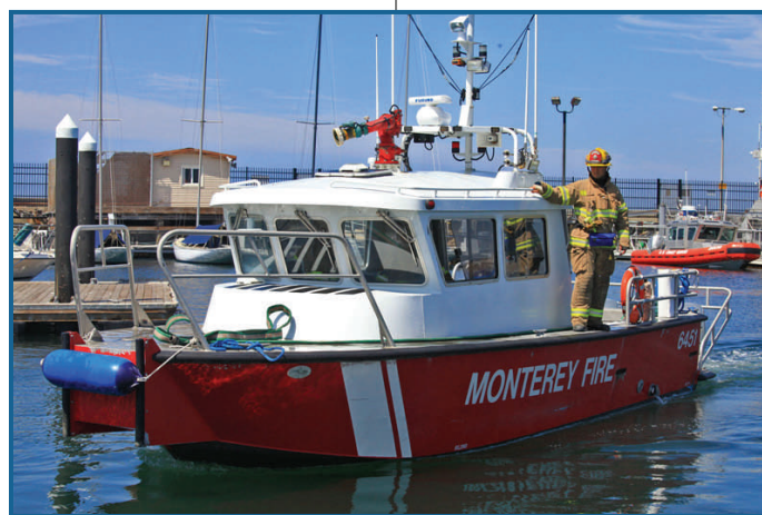
The Pearl - 6451 is located at the Coast Guard Pier. It is powered by twin 125 horsepower Honda outboard engines and a 1500 GPM pump. It is equipped with GPS, radar and two radios. The Fire Boat is crossed manned by Engine Company 6412 Stationed in New Monterey.
